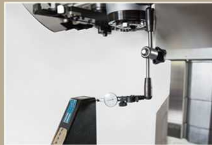
Vertical straightness of Y&Z axis
