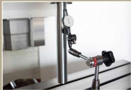
Spindle run-out check
