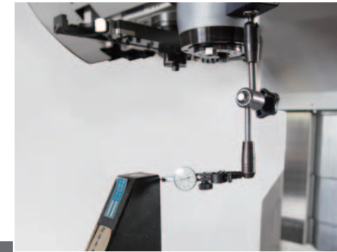
Y, Z axis vertical adjustment
