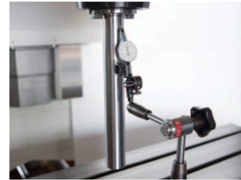
Spindle run out inspection test
